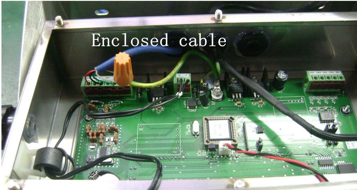
The TI-1520 indicator contains a connection terminal on the main board for connection to the load cell cable. Connect your shielded load cell cable (not included) to the appropriate terminal on the main board. **NOTE:** 6-wire connection is optional.
