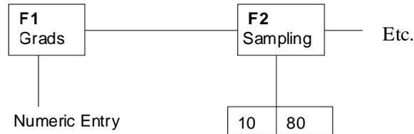
1. To move to a new heading, use the TARE (left) or PRINT (right) key to move right or left in the Menu.
