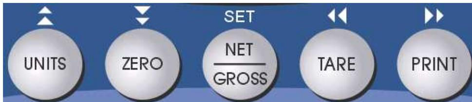
4. After setting the exact value, press the NET/GROSS key to save the ID Number value. The display will show "**SET**" momentarily, and then revert back up to A8.
